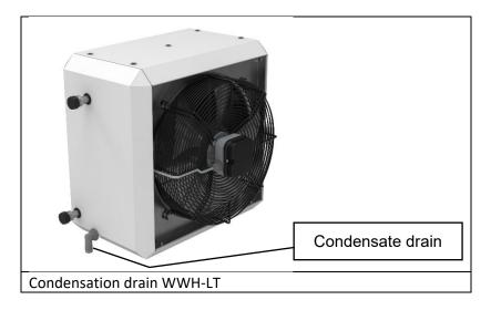
**Wall setup:** The pipe connections for water should always be **horizontal**, with a view to venting of the internal pipes. The heater can be turned over slightly, but the heater may absolutely not hang askew. Place the heater in such manner that, the return connection (cold water) is at the lowest point. It's important to place the venting in the duct near the heater.
