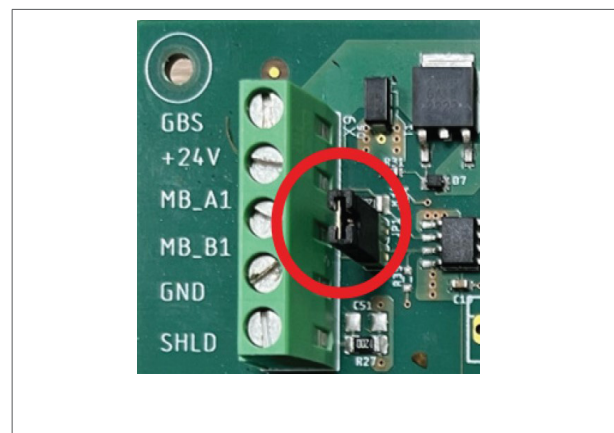
Figure 12 - Jumper to connect the 120Ω end terminal
